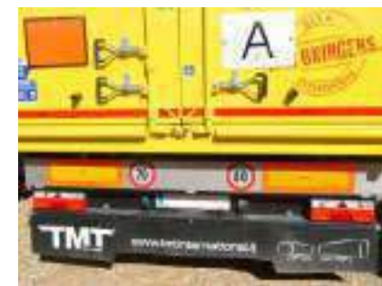
• Foldable "A" waste transport sign German model • Pneumatic safety lock on rear doors
