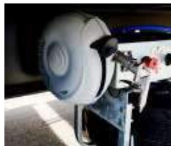
Compressed air quick coupling with the gun and hose in the rear part of the vehicle for cleaning the loading floor
