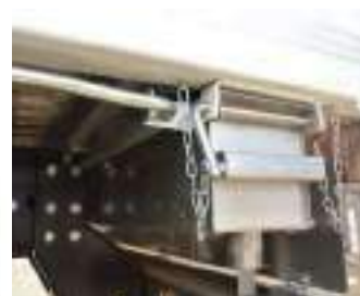
Semi-waterproof moving floor with 21 slats with rear water collection tank of about 50/300 liters with side discharge
